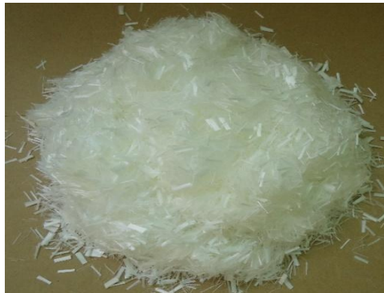
Figure 1 REC15x8mm PVA fibers
