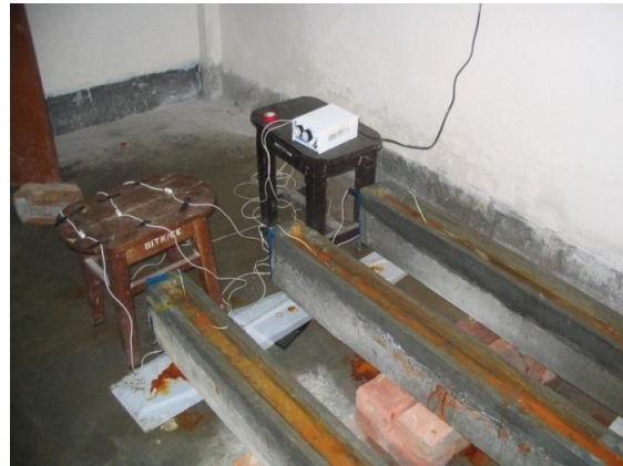
Figure 3: Test setup for accelerated corrosion
