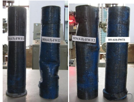
Fig. 3 Failure modes of Full wrapped specimens
