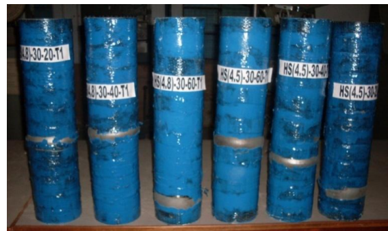
Fig. 4 Failure modes of Strip wrapped T1 columns
