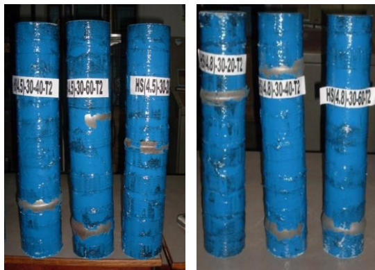
Fig.5 Failure modes of Strip wrapped T2 columns
