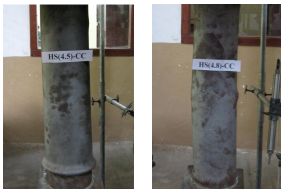
Fig. 2 Failure modes of Control Columns
