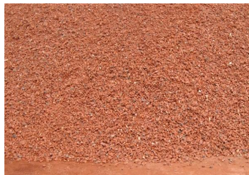
Figure 1: (a) Physical appearance coarse aggregate
