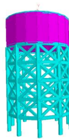
Figure-6 Staging with crossbracing staging
