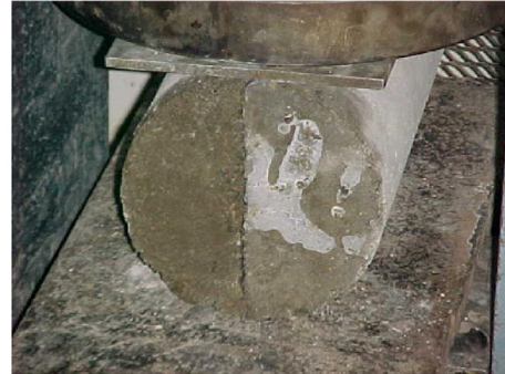
Fig. 2 Cylindrical splitting specimen at failure
